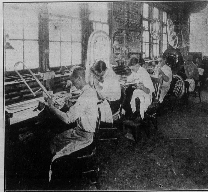
After being removed from the plating bath, instruments are sent to the burnishing department, where the high mirror finish or "burnish" is given to the bell and certain portions of the body of the instrument. This is all skilled hand work, and many striking effects are achieved by the craftsmen. (See last column, page 9.)
